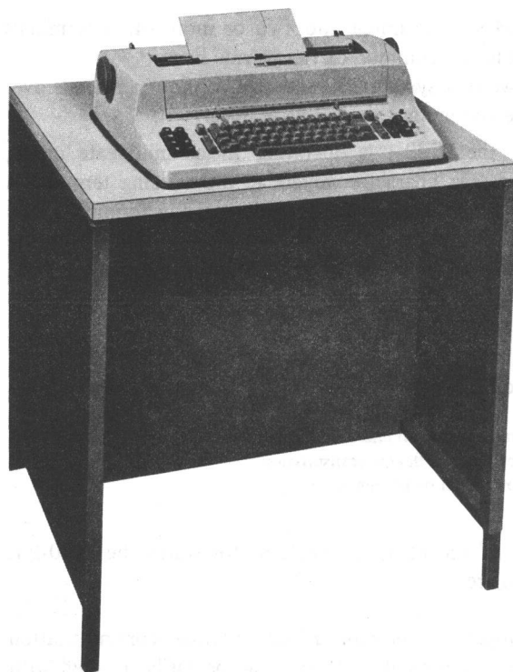
Figure 8-11. IBM 2740 Communication Terminal Model 1
