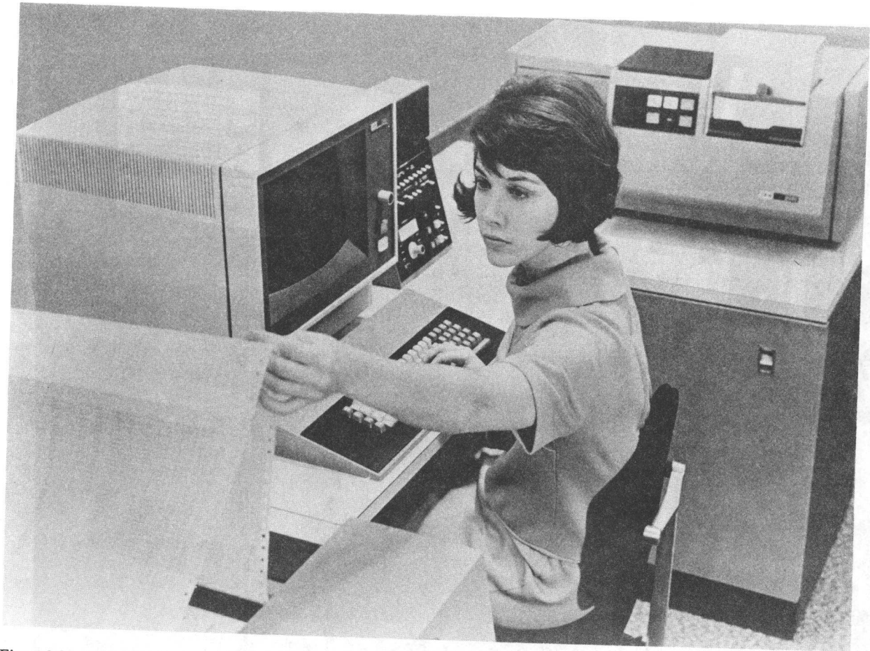
Figure 8-27. IBM 2770 Data Communication System
