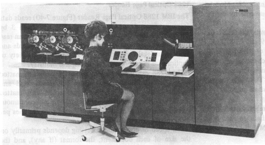
Figure 7-37. IBM 1287 Optical Reader Model 5
