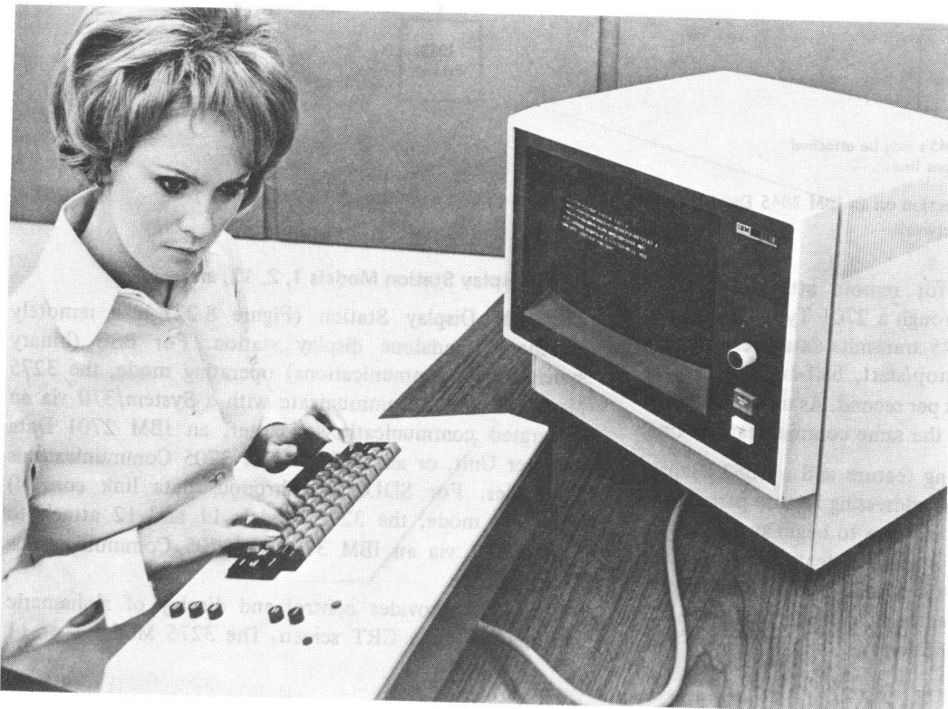
Figure 8-20. IBM 2265 Display Station with Alphameric Keyboard
