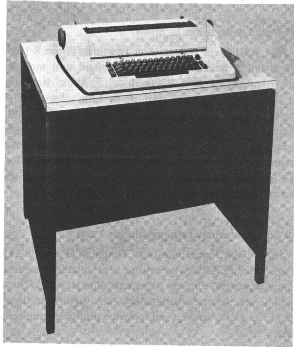
Figure 8-12. IBM 2741 Communication Terminal
