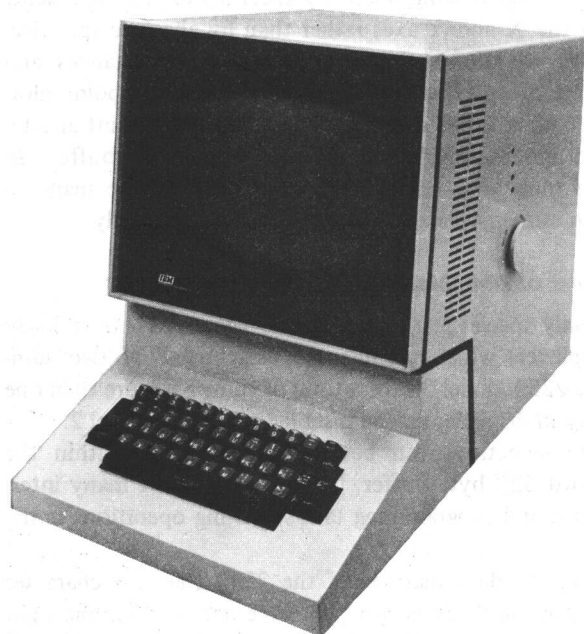
Figure 7-21. IBM 2260 Display Station with an Alphameric Keyboard
